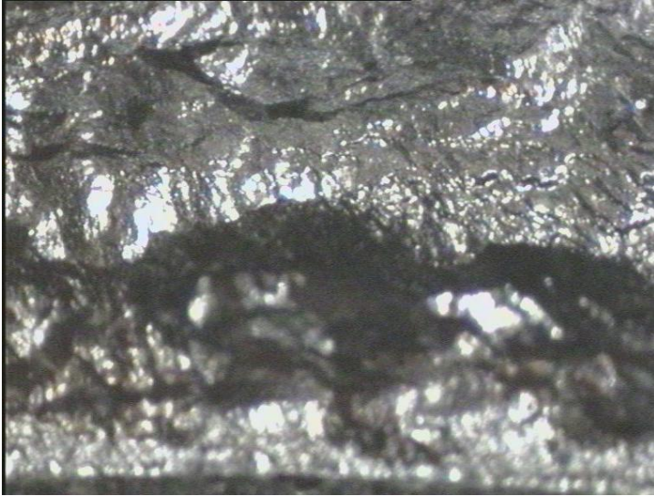
Figure 3 Severe adhesive wear that occurred between the end coil and first active coil of a spring made from 5mm diameter 17/7PH after two years of almost continuous service in a diesel engine. Note the rough topography and lumps that have been ripped from the wear surface and the cracks at the top of the photograph, which form prior to the ripping out.
