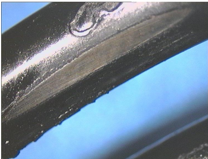
Figure 2 Abrasive wear at the inside surface of a painted torsion spring where it had made contact with its mandrel. There is little red-brown discoloration in the wear, which is fretting oxide, which has formed despite the excellent lubrication of this spring, which failed due to an ordinary fatigue mechanism after 140 thousand cycles.
