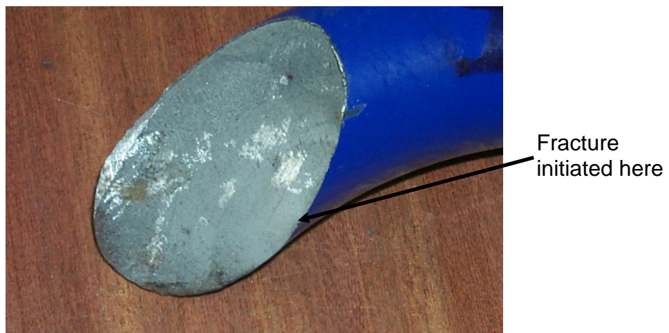
Figure 1 Helicoidal shaped fatigue and overload fracture.
