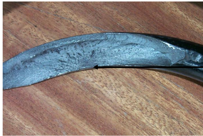
Figure 5 A longitudinal split is a consequence of the fatigue crack and not its cause.
