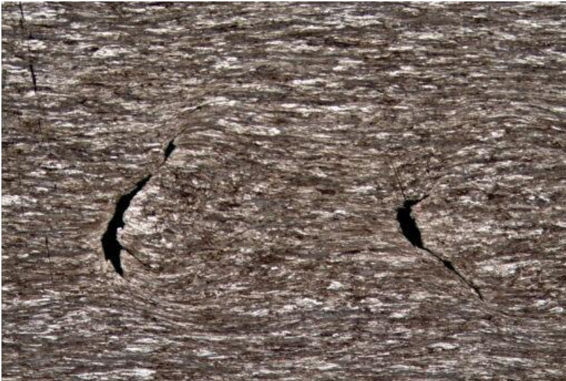
Figure 1 Over-drawn music wire with chevron shaped cracks along the centre line.
