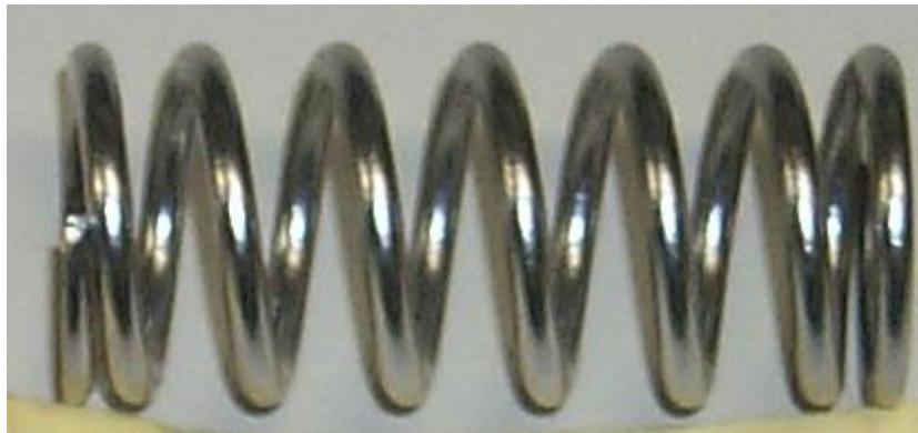
Figure 4 17/7PH spring, peened and electropolished
