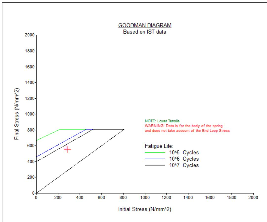
Figure 1 Goodman diagram for the body of an extension spring operating at 6 Hz and 12 Hz
